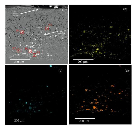
**Fig. 2.** Image of a cross section of a thallus *Peltigera aphthosa*, obtained in the mode of detecting backscattered electrons (a) and element distribution maps: (b) Al, (c) Fe, (d) Si. Areas with bright colors correspond to the maximum content of the element; UC—upper cortex, M—medulla; the elemental composition of mineral particles (P1–P5) is given in Table 2.
