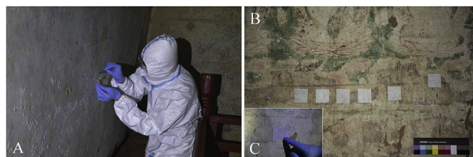
Fig. 2. Microbial deterioration of wall paintings and its control. A: Whitish fungal outbreak investigation and samples collection at the World Cultural Heritage Site Maijishan Grottoes, Tianshui, China; B and C: Soft fiber papers infiltrated with screened biocides for controlling of brownish microbial spots causing deterioration on wall painting of Mogao Grottoes, Dunhuang, China.
