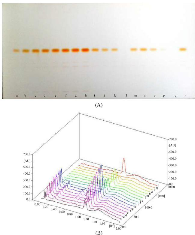
FIG. 1. Biodecolorization analysis of OERL by lichen *Parmelia* sp. (A) Ascendingly developed TLC plate with standard concentrations (lanes a–h), samples exposed to different pH (lanes i–m), samples exposed to different temperatures (lanes n–r), (B) scanning spectra of the same samples showing increasing peaks with increasing concentrations of standards and reduced peaks at optimum experimental conditions.
