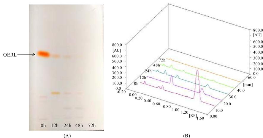
FIG. 3. Time dependant decolorization of OERL. (A) Developed plate with OERL at 0, 12, 24, 48 and 72 h. (B) Scanning spectra of same plate showing gradual reduction in peaks of OERL after biodecolorization by lichen *Parmelia* sp.
