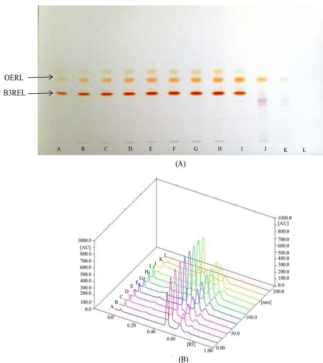
FIG. 2. Biodecolorization of dye mixture containing two different dyes OERL and B3REL. (A) Developed TLC plate with standard concentrations of both dyes (lanes A–I) and decolorized samples after incubation of 24 h (lane J), 48 h (lane K) and 72 h (lane L). (B) Scanning spectra of the same plate showing increasing area of peak as per increasing concentrations of standards and reduced peaks after biodecolorization.
