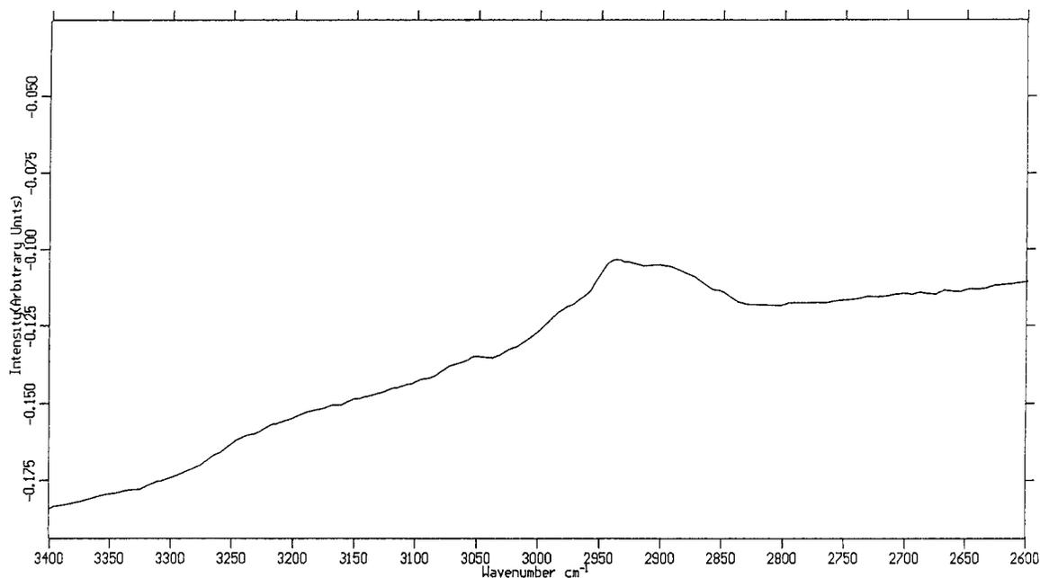
**Figure 4.** FT Raman spectrum of the lichen encrustation of *Diploschistes scruposus*; samples removed from colonies on outer walls of the Convento de la Peregrina. 1064 nm excitation,  $8\text{ cm}^{-1}$  spectral resolution, 4000 scans accumulated, wavenumber range  $2600\text{--}3400\text{ cm}^{-1}$ .
