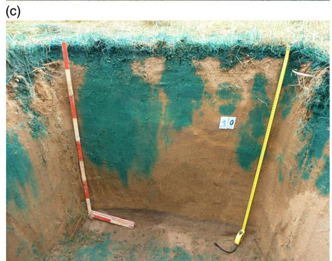
**FIGURE 7** The image of vertical sections of dyed soil, taken in (a) pure sand with a negligible impact of vegetation or organic matter at site S0; (b) sandy soil covered with biological soil crust at site S1; and (c) sandy soil covered with grass at site S3
