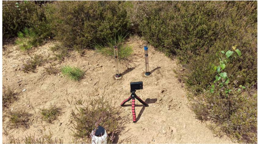
**FIGURE 1** The pairwise arrangement of minidisk infiltrimeters for measurements of water (right) and ethanol (left) infiltration at Mehlinger Heide, Germany
