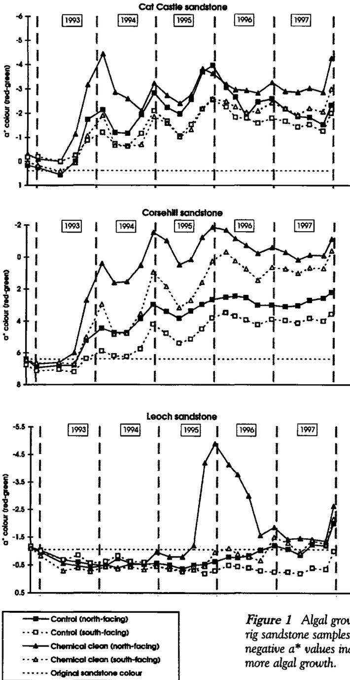
*Figure 1 Algal growth on test rig sandstone samples. More negative  $a^*$  values indicate more algal growth.*
