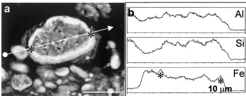
**FIGURE 5** SEM-BSE image (a) of a fossilized Antarctic endolithic microorganism cell (scale bar = 5  $\mu\text{m}$ ) and its Al, Si, and Fe composition shown by the EDS microprobe scan-line profile (b) along the white arrow drawn in Figure 5a; asterisks indicate the cell wall zone rich in Fe.
