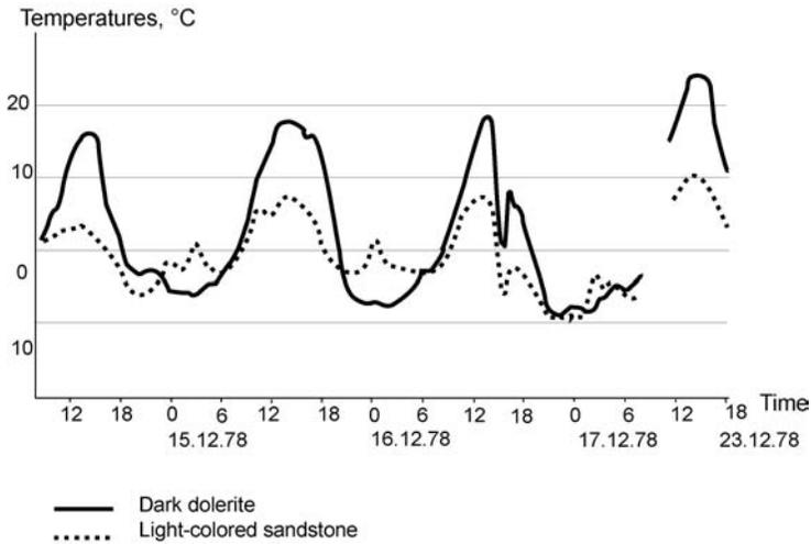
**Fig. 3.** Subsurface temperatures recorded at  $-1$  cm on rock surfaces facing north in the Darwin Mountains, Antarctica,  $80^{\circ}$  S: dark dolerite vs. pale sandstone (after Miotke and Hodenberg, 1983, Fig. 17, p. 116, modified).
