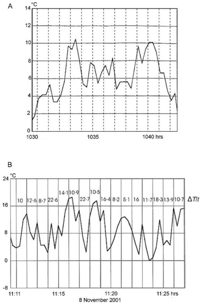
**Fig. 6.** Short-term and large-magnitude  $\Delta T/\Delta t$  events at the surface of pale rock types in the Antarctic Peninsula region. A. Light-colored arkosic sandstone at Two Step Cliffs, Alexander Island (from Hall, 2003, Fig. 4, p. 351). B. Light grey granodiorite at Rothera Point, Adelaide Island (from Hall and André, 2003, Fig. 5A, p. 833).
