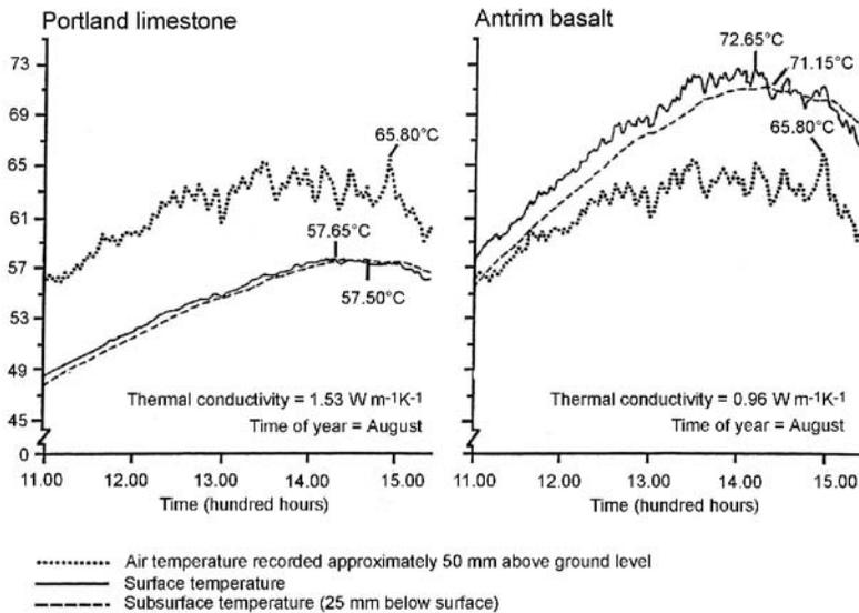
**Fig. 2.** Air temperature and simultaneous surface and subsurface temperatures of white Portland limestone and dark Antrim basalt recorded in August 1992 at Badwater, Death Valley, California (Warke, 2000, Fig. 2, p. 90).
