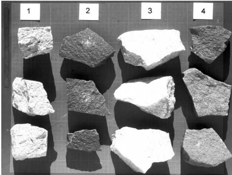
**Fig. 1.** Sandstone samples of various colors from Two Step Cliffs, Alexander Island (West Antarctica). From left to right: 1 = sound pale sandstone; 2 = sound dark sandstone; 3 = chemically whitened pale sandstone; 4 = reddish-brown Fe-rich coating due to oxidation on dark sandstone. Photo by M. F. André.
