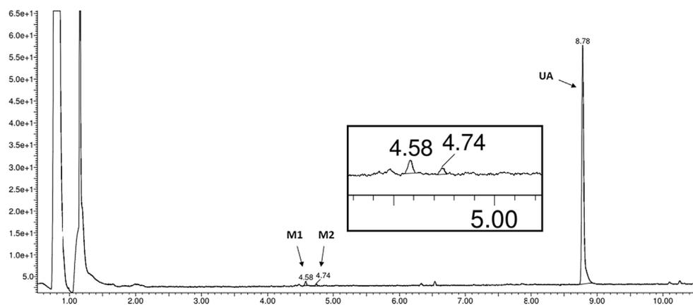
**Fig. 2.** UPLC chromatogram of the sample from the incubation mixture, consisting of (+)-usnic acid and glutathione in human liver microsomes. Metabolites (M1 and M2) and (+)-usnic acid (UA) are indicated by arrows. Magnified in the inset.
