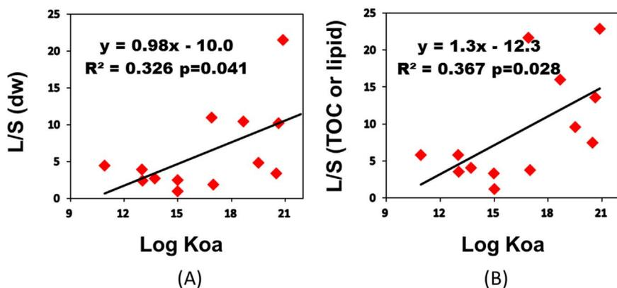
Fig. 6. The ratio of L/S in the western TP as a function of log  $K_{OA}$  for dry weight (A) and TOC/lipid weight basis (B) of PAHs at 0.5 °C (average annual temperature of the western TP (Chen et al., 2017)). The log  $K_{OA}$  is provide in Table S2.
